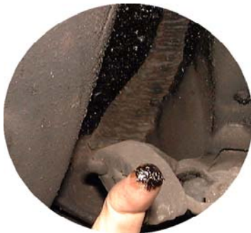
After seven years solvent free Noxudol 300 remains Soft and maintains its texture.
