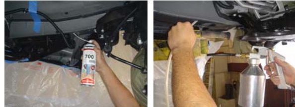
Rustproofing the interior cavities of the underfloor
