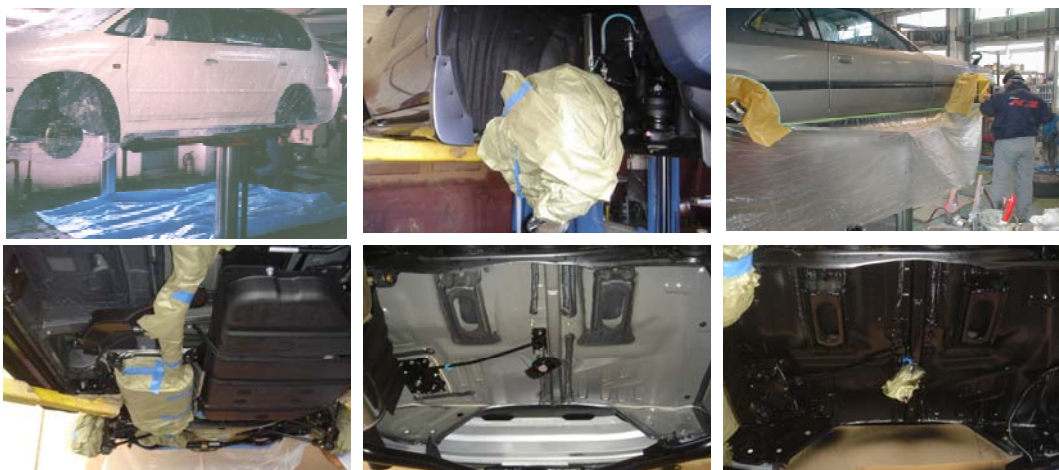
Example: On how to cover a vehicle before applying the Noxudol undercoat
